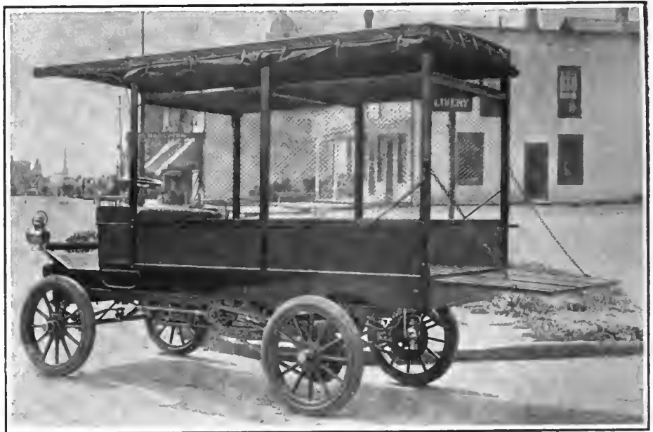
RAPID 3,000-POUND DELIVERY WAGON WITH DOUBLE OPPOSED GASOLINE MOTOR.
